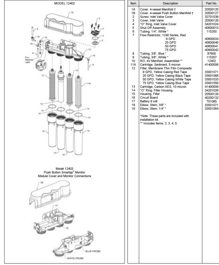
Figure 8.B: Exploded Schematic, 12402 and 12403 Model Series
