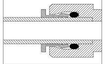
B. Tube must seat firmly at bottom of fitting.
