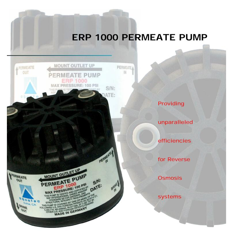
The Permeate Pump operates as a non-electrical energy recovery device which dramatically improves the efficiency of RO systems. Using only the available energy from the brine water (otherwise lost to the drain), the pump forces product water into the storage tank. This process effectively reduces membrane back pressure to less than 5 psi and allows the membrane to maximize its use of the available feed pressure.
