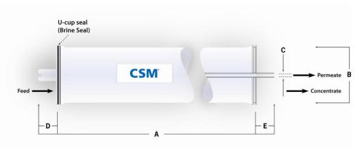
Each membrane element supplied with one brine seal, one interconnector (coupler) and four o-rings.
