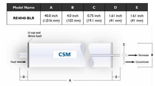
Each membrane element supplied with one brine seal, one interconnector (coupler) and four o-rings.
