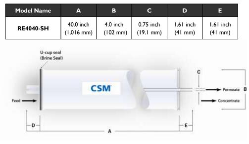
**A** = 40.0 inch (1,016 mm) **B** = 4.0 inch (102 mm) **C** = 0.75 inch (19.1 mm)
