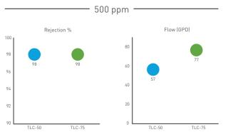
Product Tested at 65 psi; 77°F; 20% recovery; 500 ppm NaCl/RO NOTE: The data above is based on internal laboratory testing.
