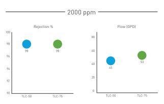
Product Tested at 65 psi; 77°F; 20% recovery; 2000 ppm NaCl/RO
