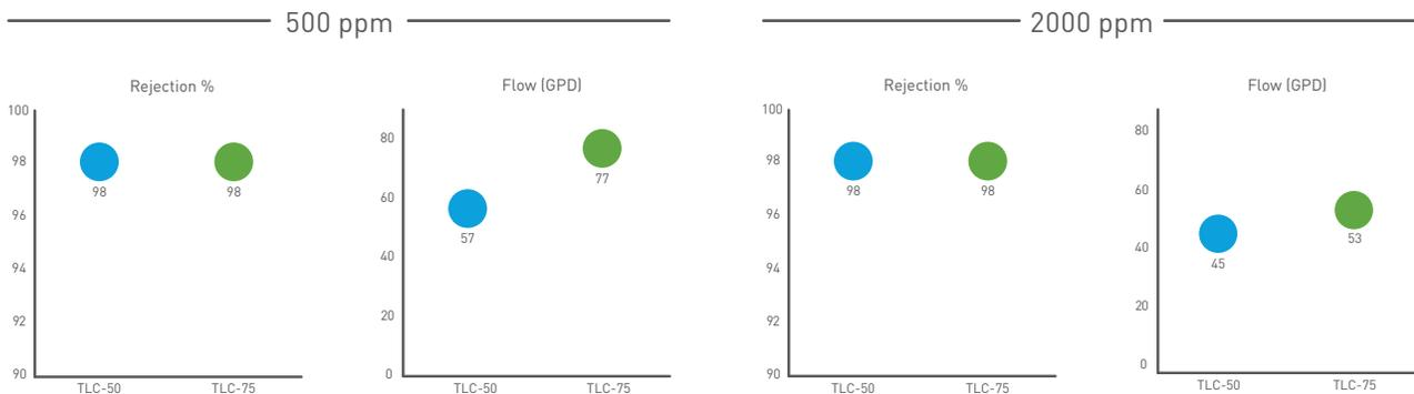
Product Tested at 65 psi; 77°F; 20% recovery; 500 ppm NaCl/RO
