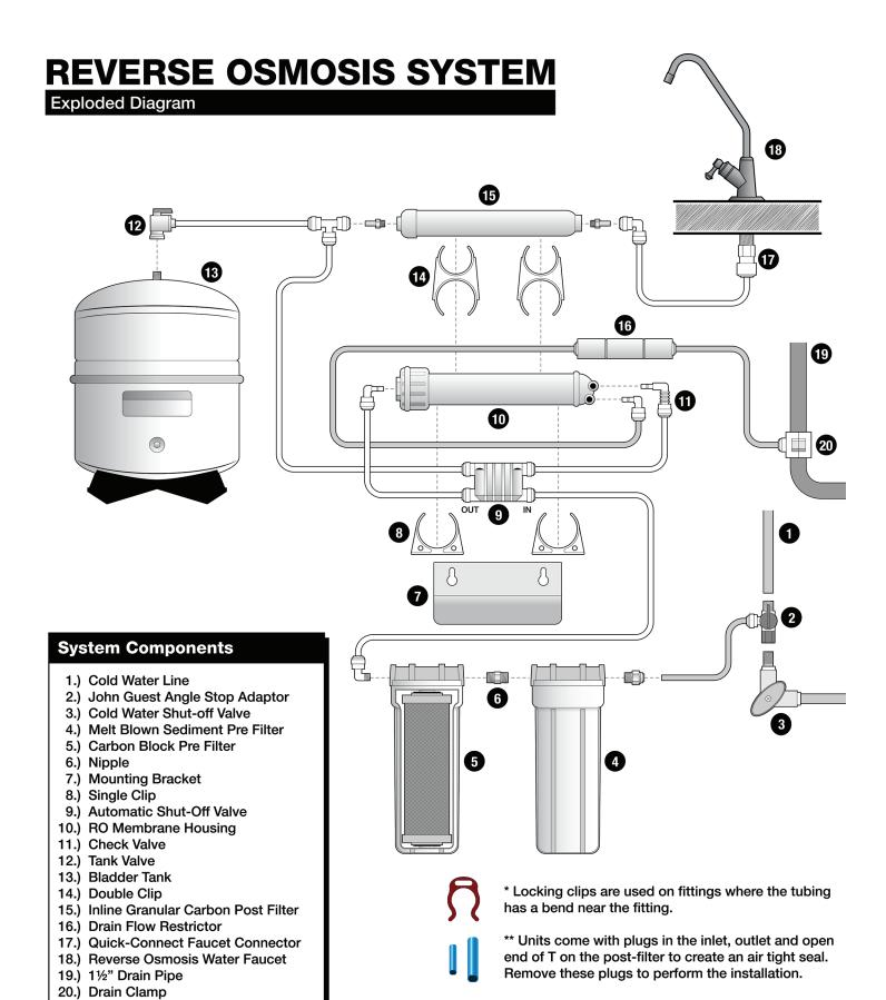
Your Reverse Osmosis (RO) System has been tested to ensure it will operate correctly. The following periodic maintenance is recommended so your system will provide years of trouble-free service:
