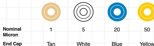
Graph colors (left) correspond with color codes (above) used to identify nominal micron rating of cartridge.
