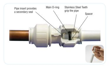
Like our Standard Fittings, Twist and Lock Fittings have a collet with stainless steel teeth that grip the pipe when fully inserted, and an O-ring to provide a permanent leak-proof seal. The additional benefit of the Twist and Lock fitting is that a twist of the screw-cap gives greater compression on the O-ring seal and locks the pipe in place for greater security.
