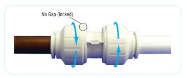
Twist the screw-cap until it touches the body flange. This locks the pipe into position and increases the o-ring seal around the pipe.
